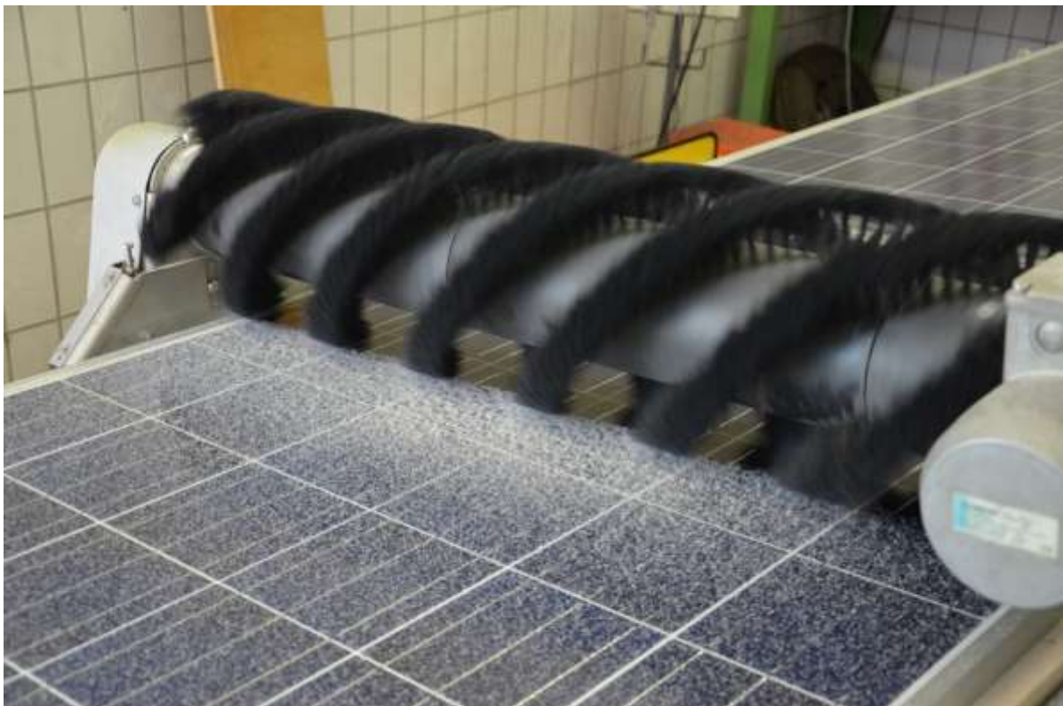
Figure 2: Dry cleaning process with the SunBrush mobil cleaning unit.
